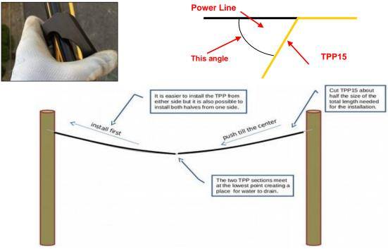
Note: TPP product is not watertight, and thus any trapped water will drip from closure joint or out of the bottom low end of TPP tube installed as pictured above. Consideration should be given to either seal and or tape up all water ingress points at open high ends of TPP pipe to reduce the amount water ingress. (Customer preferred product and methods)
