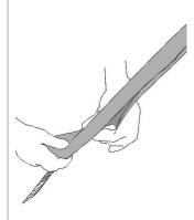
**A3.** Remove any gaps or kinks along the length of the conductor once installed.
