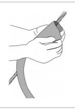
**A1.** Spread open one end of the Possum Tails and place it around the conductor.
