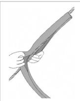
**A2.** Spreading the whole length open while installing along the conductor.
